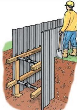
Trench sheets with timber walings, screw props, punchons and sole plates
